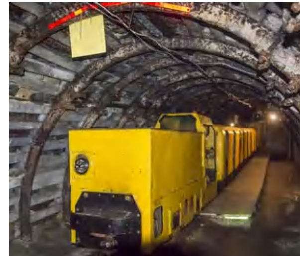
Electric traction for railway rolling stock powered by batteries
